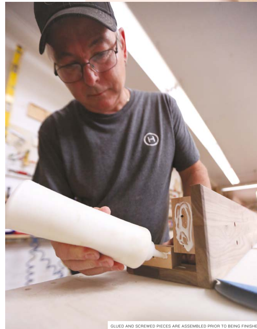
GLUED AND SCREWED PIECES ARE ASSEMBLED PRIOR TO BEING FINISHED
